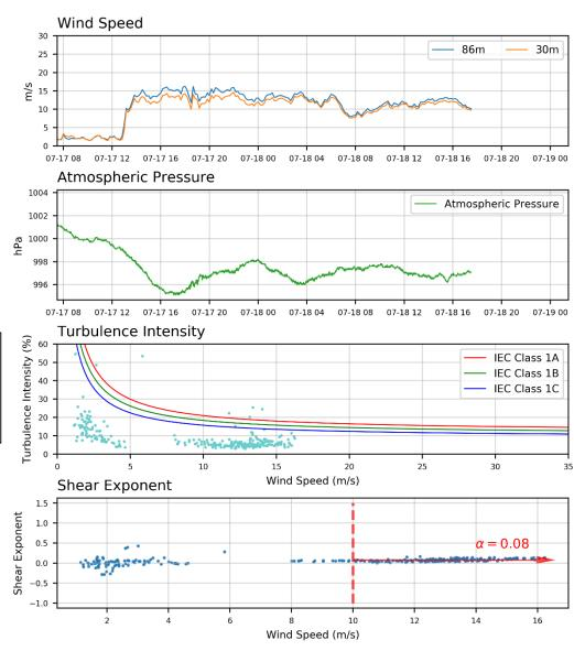
Wind data observed at 86m and 30m heights. Atm. Pressure measured at 20m height.
