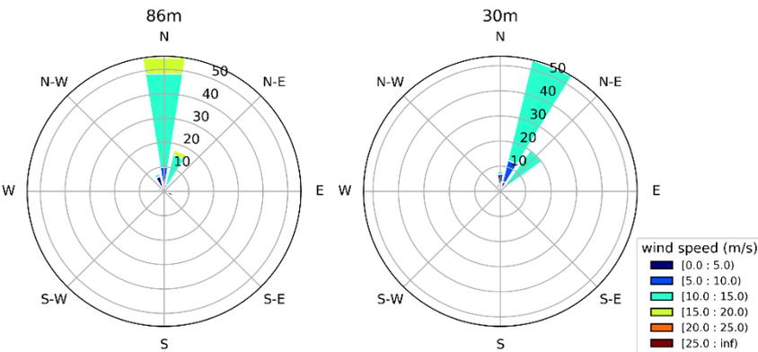
Wind data observed at 86m and 30m heights. Atm. Pressure measured at 20m height.
